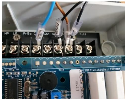
DIVERTING VALVE ELECTRIC CONNECTIONS FIG. 3-12
